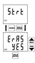
If it is needed to clear the memory before logging start, first it is necessary to select menu item logging START (symbol Strt) and confirm by pressing ENTER key.
