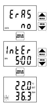
Instrument offers the possibility to clearing the instrument memory (ERAS). If you do not wish to clear the memory before new logging start, confirm selection ERAS NO by pressing the ENTER key.
