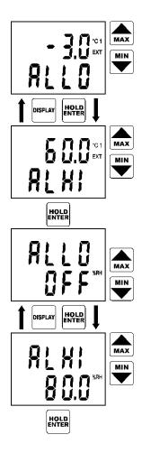
Reading ALLO indicates adjusted lower alarm limit (here air temperature). Set the desired value by means of the arrow keys. Press and hold the arrow key UP to make value increase fast. Press and hold the arrow key DOWN to make value decrease fast. Release the arrow key and press ENTER to confirm new limit.
