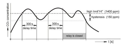
**Low limit "Lo"** – the relay closes when measured value falls below preset "low limit" for longer time than preset "delay time". Relay goes open when measured value exceeds "low limit" value plus the "hysteresis" value. See example.
