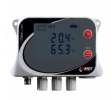
The Datalogger is designed to record temperature for four external Pt1000 probes. In case of exceeded set limits, SMS and JSON messages can be sent via GPRS data connection. It is possible to set the regular sending of JSON messages to COMET Database, the sending interval is adjustable.
