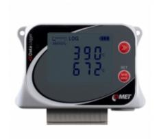
The Datalogger is designed to record temperature for four external Pt1000 probes. In case of exceeded set limits, SMS and JSON messages can be sent via GPRS data connection. It is possible to set the regular sending of JSON messages to COMET Database, the sending interval is adjustable.
