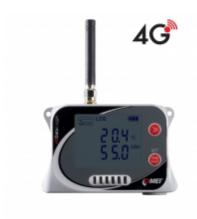
4G datalogger is designed to record temperature and humidity from built-in sensors. In case of exceeded set limits, SMS and JSON messages can be sent via GPRS data connection. Measured values can be sent to the internet storage <a href="COMET Cloud">COMET Cloud</a>, which is a complete monitoring, alarm and analysis system.
