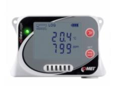
Datalogger is designed to record temperature, humidity and CO2. In case of exceeded set limits alarms are indicated by LED, LCD and acoustically by built-in beeper.
