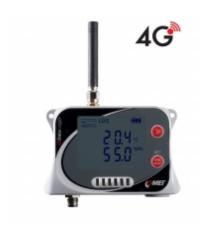
4G datalogger is designed to record temperature and humidity from built-in sensors and temperature from external probe. In case of exceeded set limits, SMS and JSON messages can be sent via GPRS data connection. Measured values can be sent to the internet storage <a href="COMET Cloud">COMET Cloud</a>, which is a complete monitoring, alarm and analysis system.
