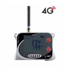
4G datalogger is designed to record temperature, humidity, atmospheric pressure and CO2. In case of exceeded set limits, SMS and JSON messages can be sent via GPRS data connection. Measured values can be sent to the internet storage <a href="COMET Cloud">COMET Cloud</a>, which is a complete monitoring, alarm and analysis system.
