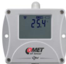
The W0911 sensor with LoRaWAN network output measures temperature [from an external Pt1000 probe on the cable](#) and can be installed directly in the measured environment thanks to its IP65-rated enclosure. LoRa devices are powered by a replaceable battery with a lifespan of up to 10 years (3 years standard).
